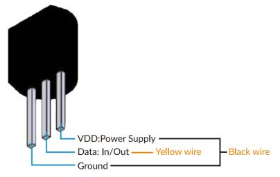
DS18B20+Sensor Element wired in parasitic power mode as shown in the diagram
