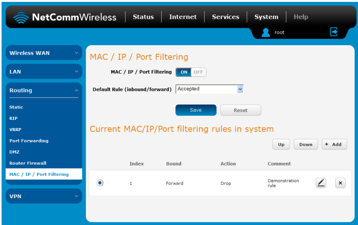
Figure 49 - MAC / IP / Port filtering
